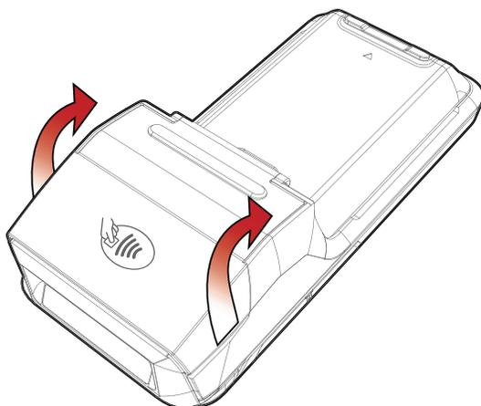
2. Referring to Figure 12, put the paper roll into the printer in the correct orientation.
